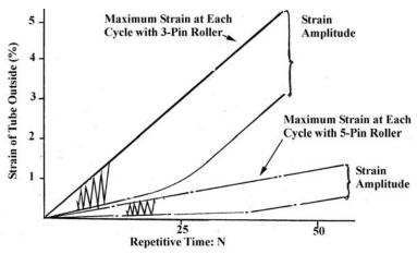
**Figure 2 Tube outside strain amplitude VS Frequency** (*Adapted from U. S. Patent No. 4,142,581, Issued March 6, 1979 to Yuji Yoshitomi and others*)
